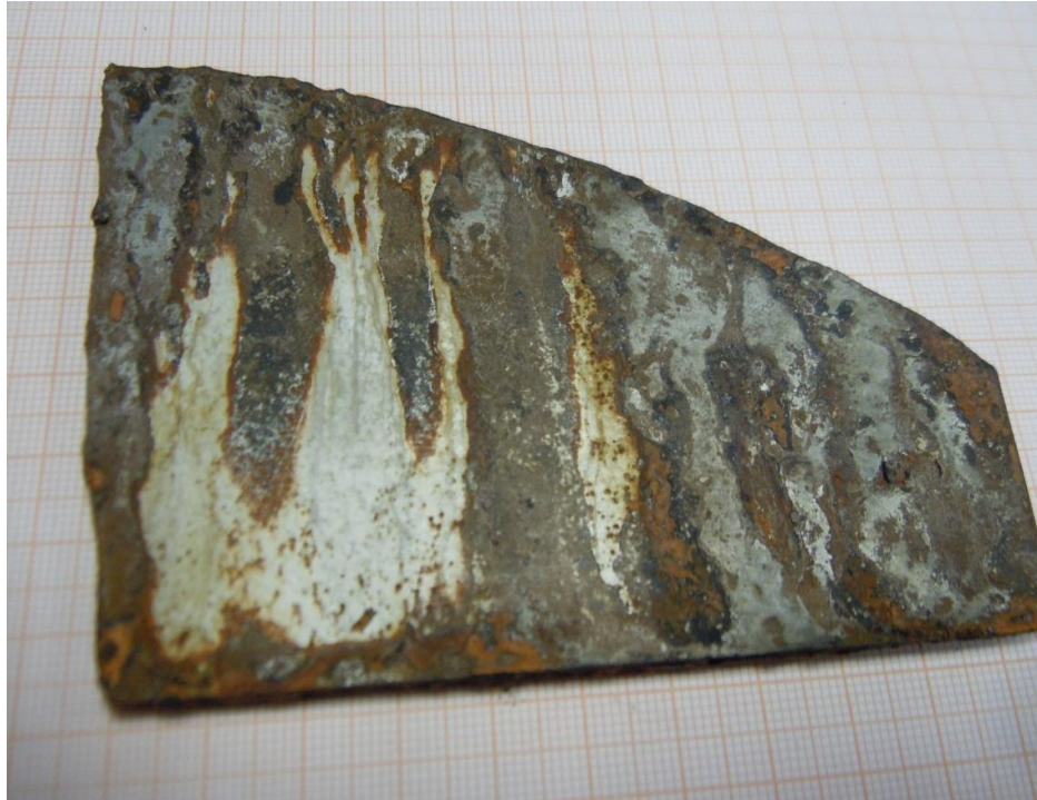
Test plate 2 - Here failure from the edges has caused most of the MM30 to fail, as expected. The ensuing corrosion covers most of the sample.
