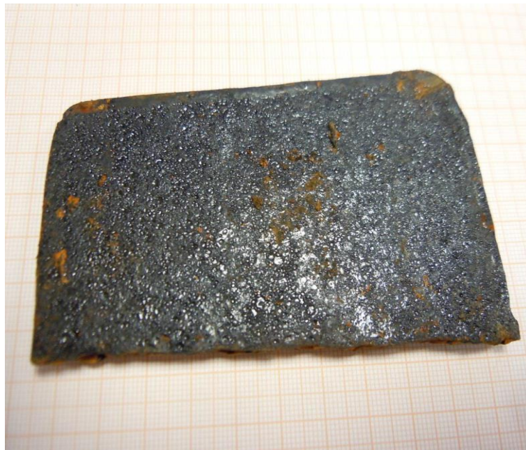
Test plate 3 - Perhaps the most interesting. It is very slightly better than sample 1. It indicates that there has been a little benefit from shot blasting. As with 1 the corrosion from the edge is unimportant, showing only the importance of profiling steel edges correctly.
